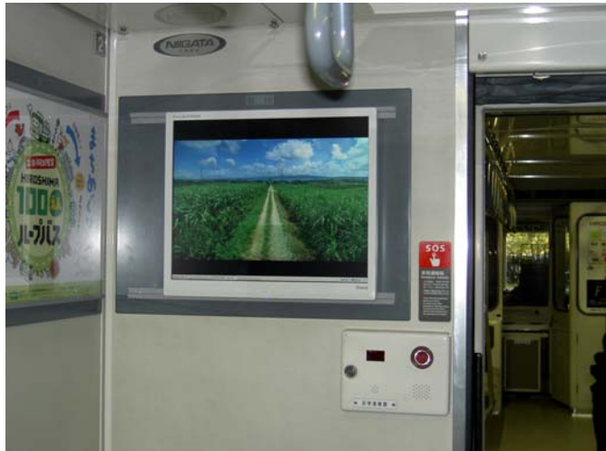
Digital signage devices installed in Astram Line cars
