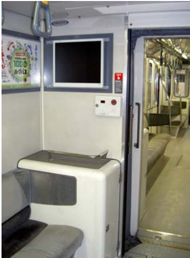
Digital signage devices installed in Astram Line cars
